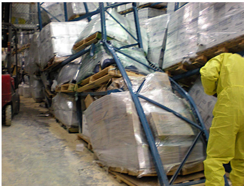
Failed and collapsed storage meant mingling of goods with unknown consequences.
